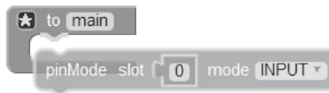
Figure 10.25 Connecting blocks together. Source: Cisco.
